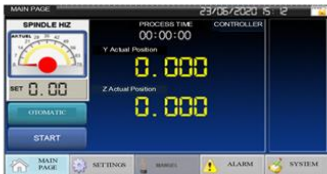
Figure 6. The main page of HMI in automatic status
