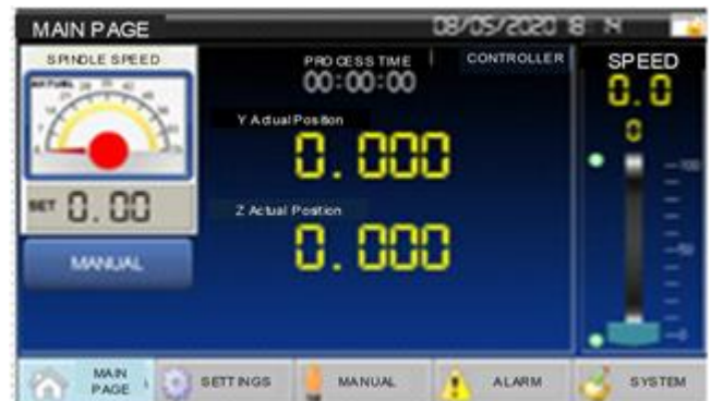
Figure 5. The main page of HMI in the manual status
