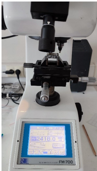
Figure 3. Coating Layer Microhardness Test Photograph.
