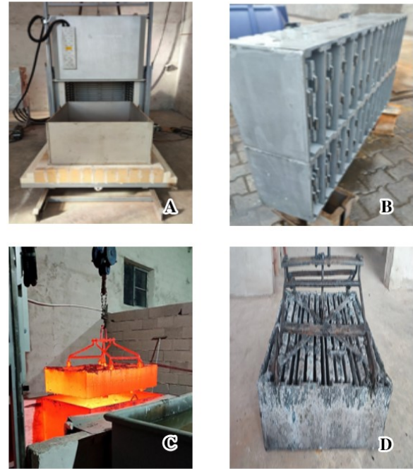
Figure 1. Coating operations of bimsbeton mold A. Coating oven and ladle B. Bims block mould before coating C. Bims block mould coating photo D. Bims block mould after coating
