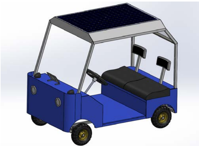
Figure 4. 3D Isometric view of the tour cart model designed in SolidWorks.
